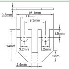
Two ways, 9.3mm pitch, compatible with the BE 2.5mm<sup>2</sup> series.
