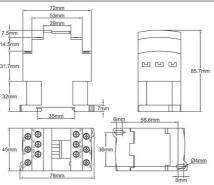
$3 \times 25A$  or  $3 \times 32A$  250/400VAC res. (AC1), screw terminals, 240VAC or 400VAC coil. Comply with IEC947-1 (EN60947-1) standard, but its large footprint limits its applications inside control boxes. It does not fit the Y8 types, but can be used in Y6 and Y7 with single pole thermostat.
