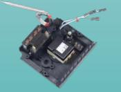
Relay 1 × 30A on thermostat extended front board, with single pole thermostat
